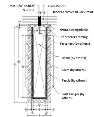
FIGURE 2 - PERIMETER DETAIL BETWEEN ADJACENT GLASS PANELS (except for silicone, dimensions are shown for illustrative purposes only)
