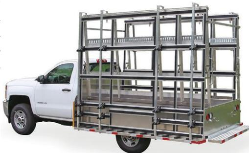
MyGlassTruck.com offers a version of its Atlas truck body for single rear wheel pick-ups with a cab-to-axle between 56 inches and 60 inches. It features a galvanized steel frame, exterior racks with five-inch usable ledges and interior racks for added capacity. Available in nine-foot and ten-foot lengths, the Atlas has a gross vehicle weight rating of less than 10,000 pounds and can be installed by MyGlassTruck or shipped for self-installation.
