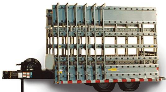
Other features include: "B" loadholding slats throughout, electric brakes on both axles, vertical interior walls and removable wheel covers. The trailer is custom manufactured and available in 10-foot to 16-foot lengths.
